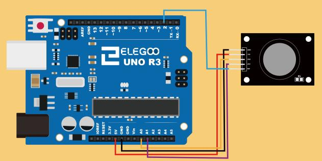
We need 5 connections to the joystick. The connections are: Key, Y, X, Voltage and Ground. "Y and X" are Analog and "Key" is Digital. If you don't need the switch then you can use only 4 pins.
