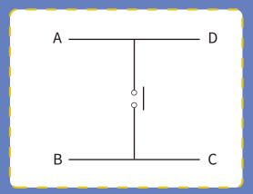
Actually, there are only really two electrical connections. Inside the switch package, pins B and C are connected together, as are A and D.
