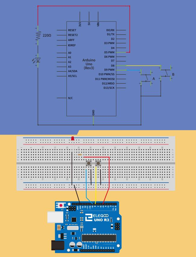
Although the bodies of the switches are square, the pins protrude from opposite sides of the switch. This means that the pins will only be far enough apart when they are placed correctly on the breadboard.
