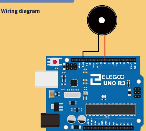
Wiring the buzzer to the UNO R3 board, the red (positive) to the pin8, black wire (negative) to the GND.
