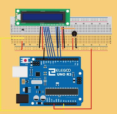
There are a few jumper wires near the pot that have been moved slightly on this layout. The 10 k $\Omega$  resistor and thermistor are all new additions to the board.
